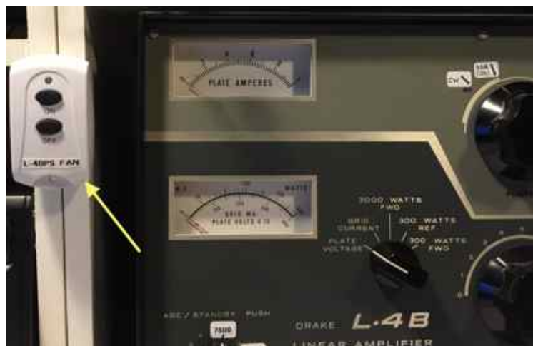
Remote fan on/off switch in place ready for use
