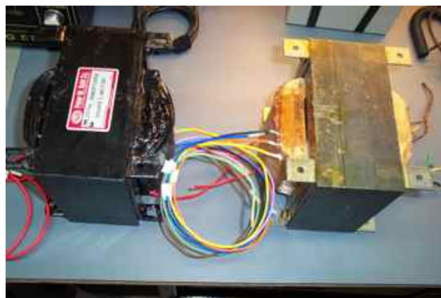
New transformer (left) and the original
