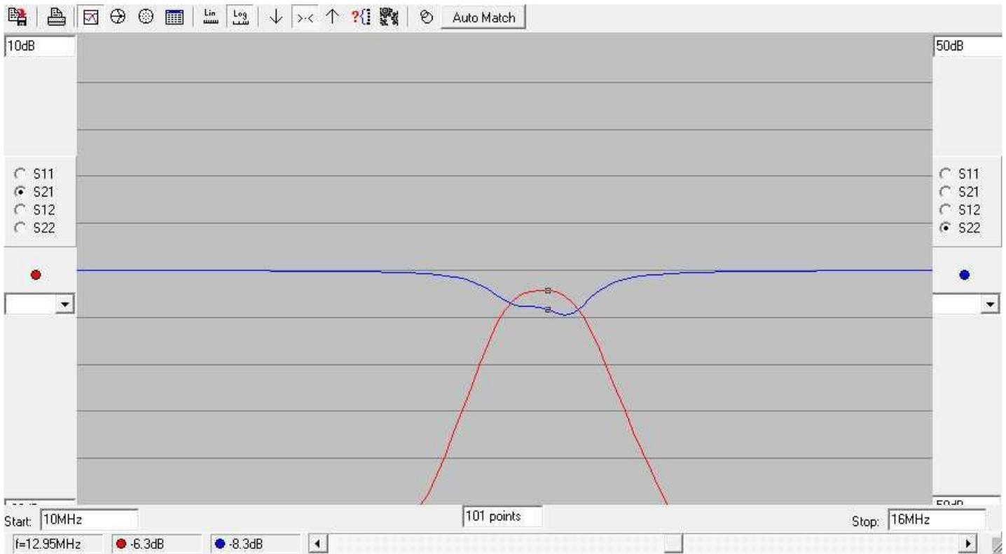
Finally, when we remove the 10k loading resistors, this is the result!
