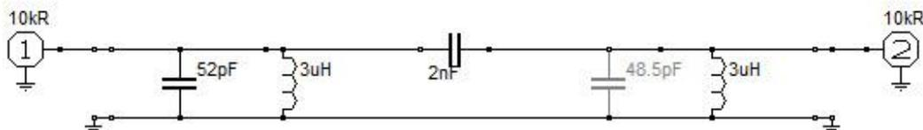
If this circuit is tuned to the frequency specified in the manual by alternately adjusting the two resonating capacitors, the passband looks like the RED trace. The marker is at 12.945 MHz, the PreMixer frequency when the receiver is tuned to 7.3 MHz:
