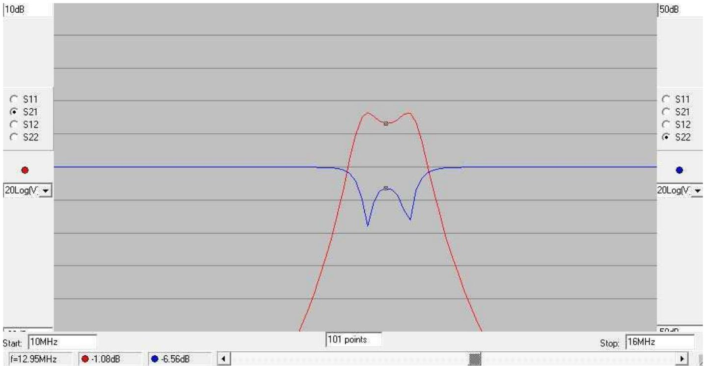
A fine adjustment of the 2 pF coupling capacitor could bring up that dip in the center, but it's only about half a dB. Not only is the top of the filter wider, the skirts are also steeper providing broader PreMixer tuning along with better spurious reduction.
