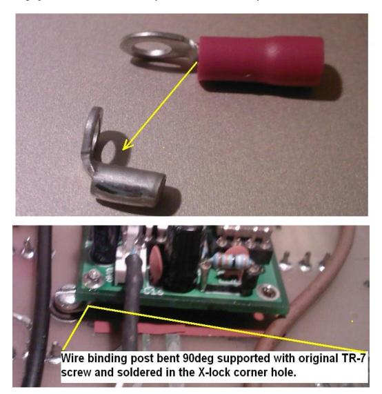
The stabilizer PCB is rather small size and supporting it by its 2 side holes gives adequate stability. A 3<sup>rd</sup> support structure at the opposite end was placed under the X-lock PCB as shown in the next picture, mainly to keep a safe distance from the TR-7 motherboard. Since the distance between the pins of the motherboard under the X-lock is rather marginal, I cut the tips of these pins flush to their solder joints and placed a layer of electrical tape over them.
