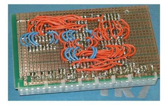
The hole spacing on the perfboard is .1" and the pin spacing on the connectors is .156". So, every other connector pin roughly lines up with one of the board holes, but even those holes had to be increased in size with a tapered diamond Dremel bit. For the pins that didn't line up with existing holes, new holes were drilled between land patterns as you see here.
