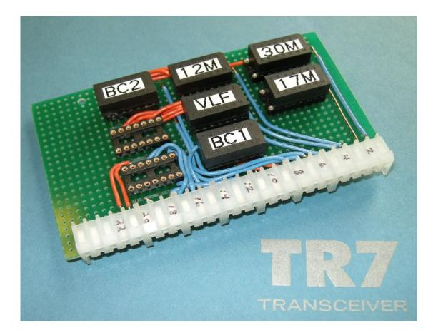
The modules require 14 pin DIP sockets, but I ran out and had to use a couple of 16 pin sockets, hence the extra socket pin positions seen on the 30 and 17M positions. Note that the overhang of the board past the connectors on the left side in the photo is not correct. I had to remove .1 inches of that so the card would fit the available clearance to the PTO housing.
