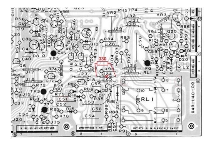
**17. Problem:** Premature 12V pilot lamp burnout. **Fix:** Reduce the pilot lamp operating voltage. Put a suitable resistor in series with the wire that supplies power to the pilot lamp terminal strip on the bottom of the radio, near the VFO. Start with approx. 20 Ohms, 0.5W. For optimum life, the pilot lamps should be operated at roughly 8 - 9V. Reducing the voltage to the meter pilot lamp requires a separate resistor of roughly 68 Ohms.
