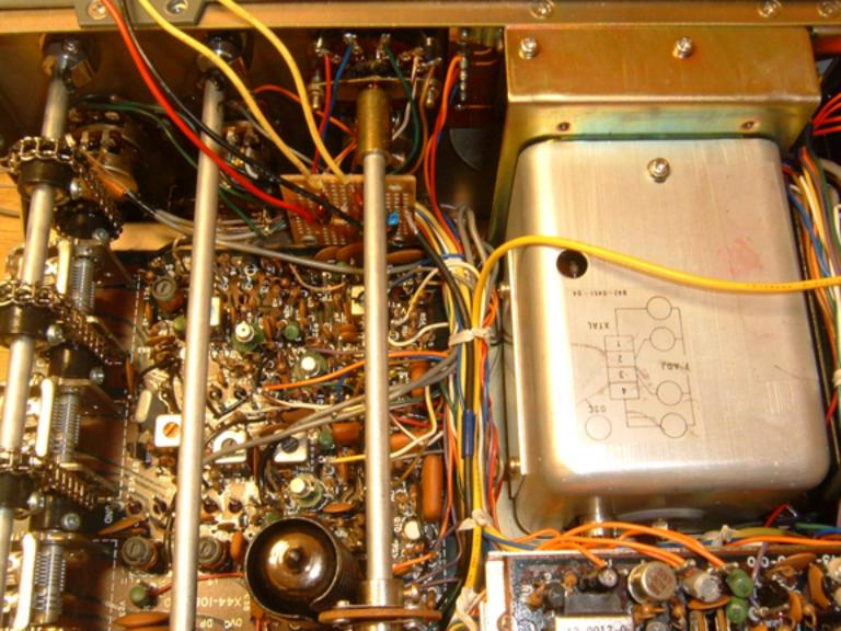
Wire soldered to 3 coils of a small spring and twisted down over the case of Q8
