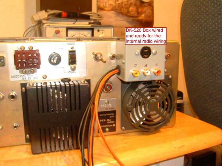
Wires for the 14 volt AC on the DC-DC terminal Board to the DK-520 Box (Orange Wires used)
