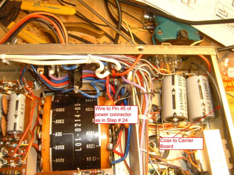
Cut Red wire to length and attach to terminal 14 on the Fix CH AVR board as shown in step #19
