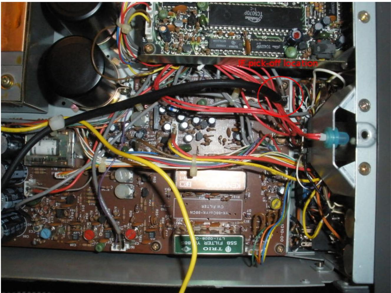
The cable then is routed towards the rear of the radio where a 3.5mm mono female jack is located. This cable is soldered and the female mono jack is mounted to the chassis below the CW KEY 1/4" female jack.
