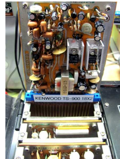
Audio balance pot is critical; If set wrong, audio is distorted
