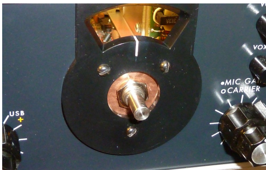
Figure 4: Escutcheon mounted to panel with copper encoder mounting sheet sandwiched between escutcheon and panel.
