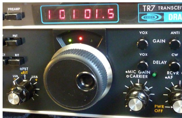
Figure 7: Finished escutcheon. The center LED is the SPLIT indicator and is yellow. The other two LEDs are for VFO-A and B and are green.
