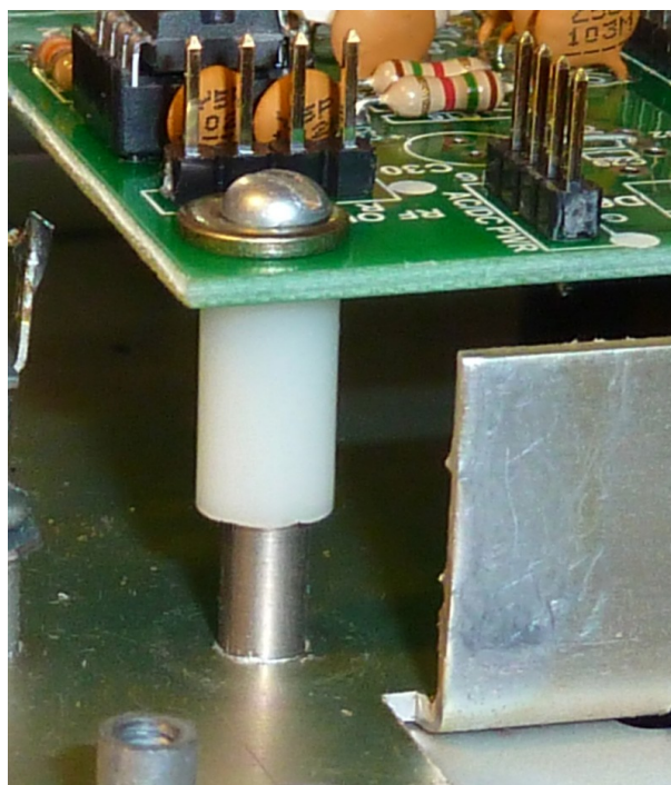
Figure 13: I used nylon spacers sitting on top of the old PTO studs for mounting the board. The studs accept 4-40 screws and these are about an inch long.
