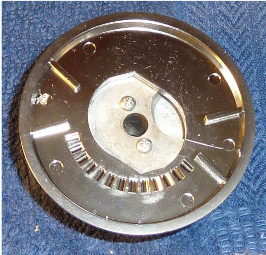
Figure 11: Rear of Tentec tuning knob as modified. Remove the two small screws and take off the friction fingers. Then glue the skirt to the knob body.
