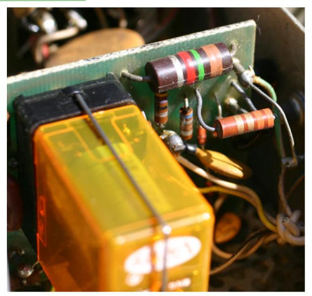
Blown and then repaired with 1/2 watt 3.3 ohm resistor.
