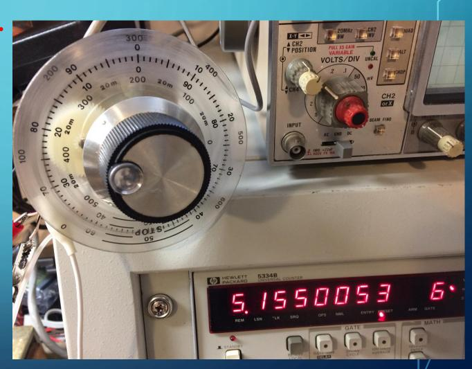
Release the idler gear train (and clamp if possible), hold the main tuning dial from moving, and rotate the dials to read 300 at the 12 clock position.
