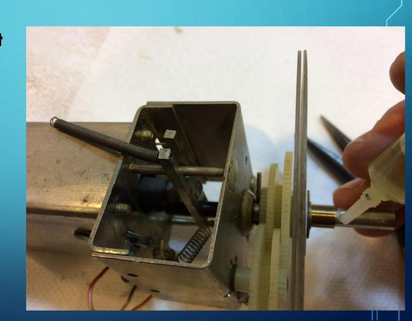
• Rotate the dials so the short end of the roll pin on the 1/4" shaft, just in front of the bearing race is pointing at the small tab on the rear of the plastic gear.
