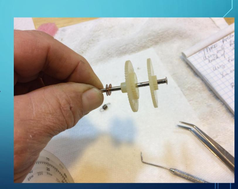
• On this style of PTO, the idler gear train and the dial assembly have to be installed at the same time to mesh the gears.
