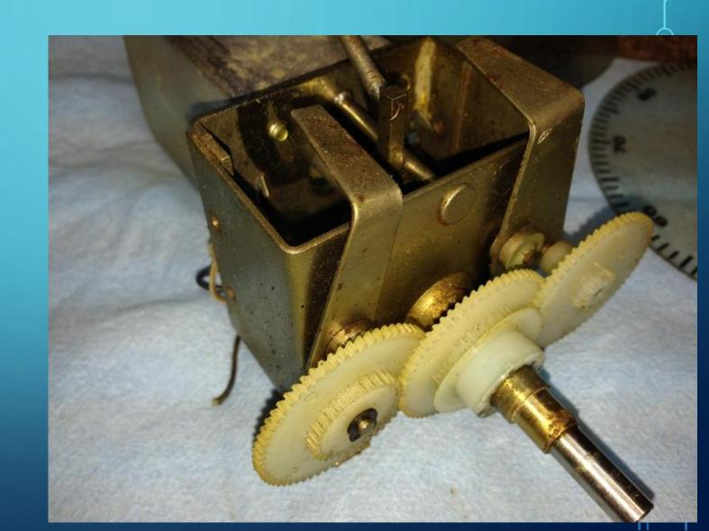
One lever, two idler trains, partially metal gear design from very late run (post 27K?) of the Cline.
