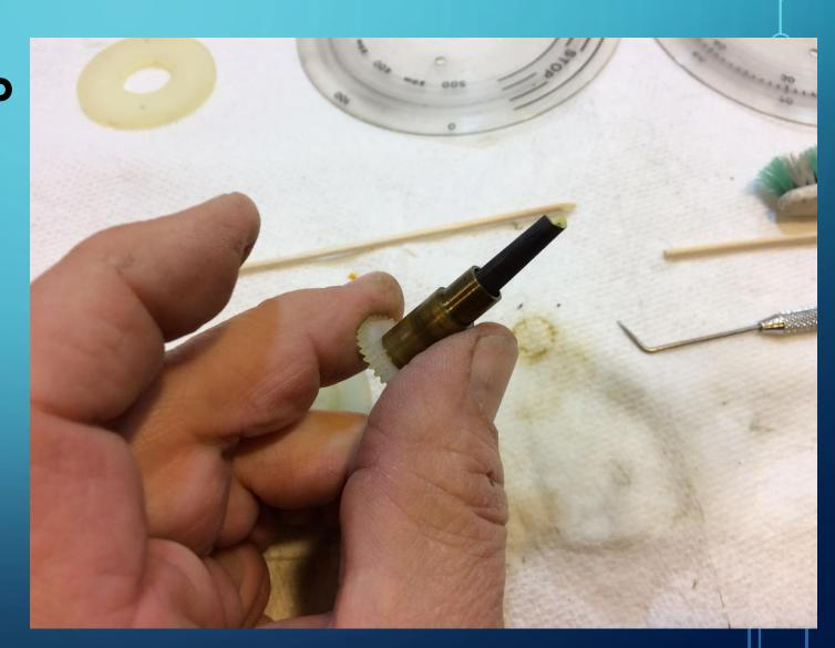
Conduct a "spin test". The brass bushing should spin easily on the 1/4"
